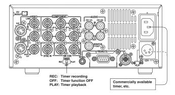
When power (AC 120 V (U MODEL), AC 220 V - 240 V (E MODEL) or DC 12 V) is supplied to this unit, it automatically enters the Record or Play mode. Using a commercially available timer, you can configure your VCR to start recording or playback at a specified time.
